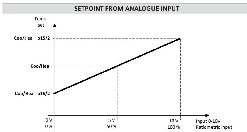
Correction calculation with ratiometric input (b20=1):
