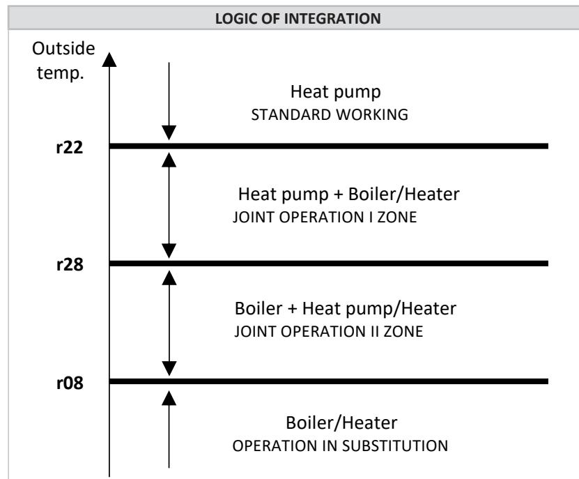
If it is necessary to change the values of the parameters, the formula  $r22 \geq r28 \geq r08$  must be followed.
