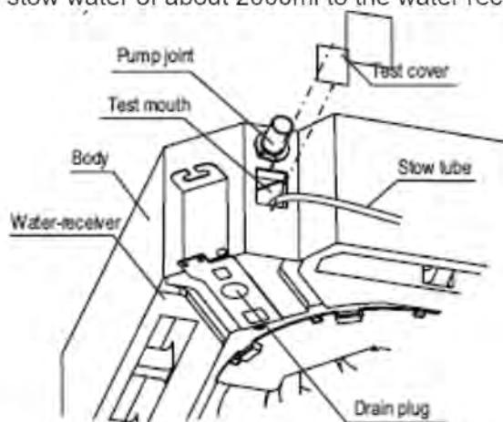
2. Turn on the power, and operate the air conditioner under the "COOLING" mode. Listen to the sound of the drain pump. Check whether the water is discharged well (a lag of 1min is allowed before discharging, according to the length of the drain pipe), and check whether water leaks from the joints.
