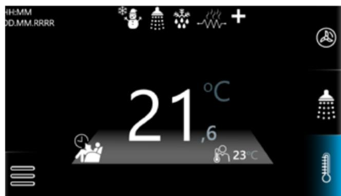
Thermostat function, which uses the e-LITE internal probe to measure the room temperature. By activating this function, the internal probe will be used to switch the heat pump on or off. The thermostat call will be sent to the heat pump if:
