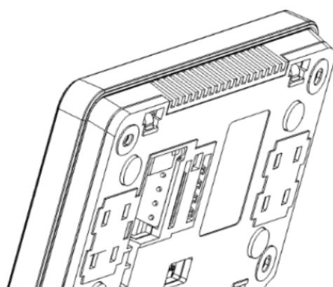
Drill the holes in the wall and use screws (max. Ø 3 mm) to fix the installation frame at the selected location on the wall. The distance of the holes can be determined by positioning the frame on the wall. Then fix the panel to the installation frame using the clips.
