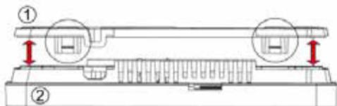
The control panel must be installed according to the instructions below. Disconnect the installation frame (1) from the back of the room thermostat housing (2). The frame is secured to the panel housing with latches. Use a flat screwdriver to detach the frame.
