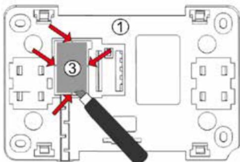
Using a sharp tool, cut holes in four places in the cover (3) for the screw terminals.
